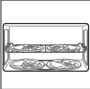
To heat 2 bottom plates together or one larger dish, the turntable should not be turning.
