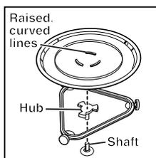
raised, curved lines in the center of the turntable bottom are between the three "spokes" of the hub.
