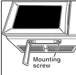
3. Remove the burnt-out bulb(s) and replace with 10W low-voltage halogen capsule bulb(s) (Part No. 8169418). Use a soft tissue to handle bulb(s), or wear a cotton glove. Do not touch bulb(s) with your bare fingers.
