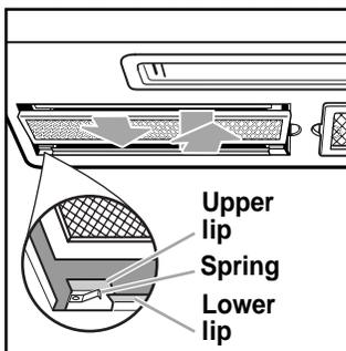
4. Soak grease filters in hot water and a mild detergent. Scrub and swish to remove embedded dirt and grease. Rinse well and shake to dry.
