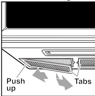
4393691), push each filter up on the side opposite the tab. Grasp the tab and slide the filter to the side. Pull the filter downward. It will drop out.
